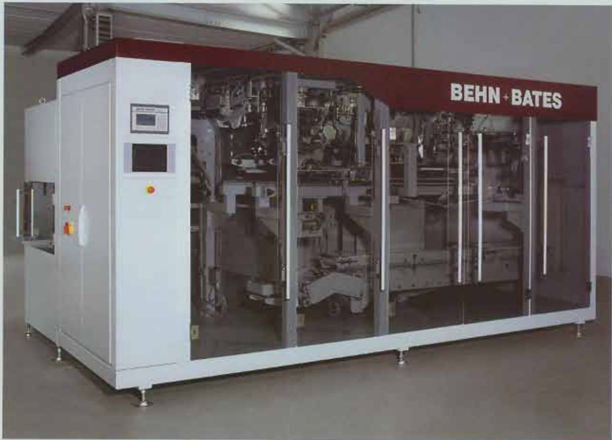
TOPLINE packing system with lateral empty bag magazine
