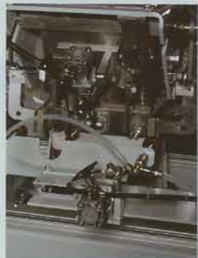
Double wall-flap filling spout with bag clamps on all sides and integrated bag deaeration
