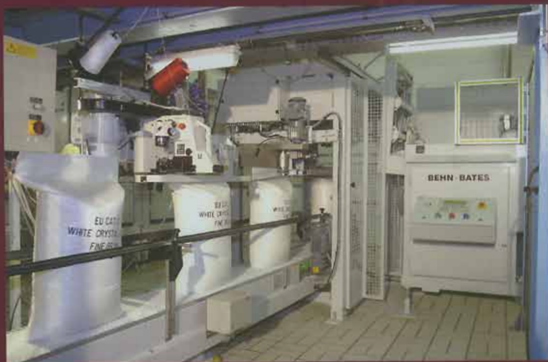
BEHN + BATES Sackomat – The high capacity packing system for open mouth bags (up to 1,200 bags per hour)
