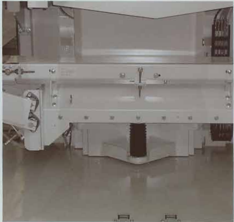
Suspended, height-adjustable bag discharge belt conveyor, even bottom for easy cleaning
