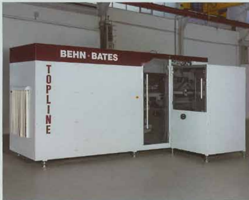
Rear view of the TOPLINE with empty bag magazine and bag placer
