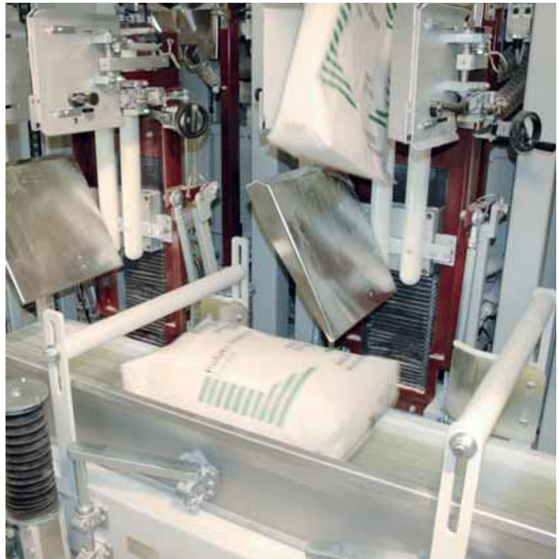
Discharge of the filled, sealed bag without any machine contamination by product dust
