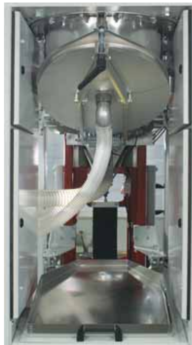
Closed filling chamber bottom with central lock and product catching tray
