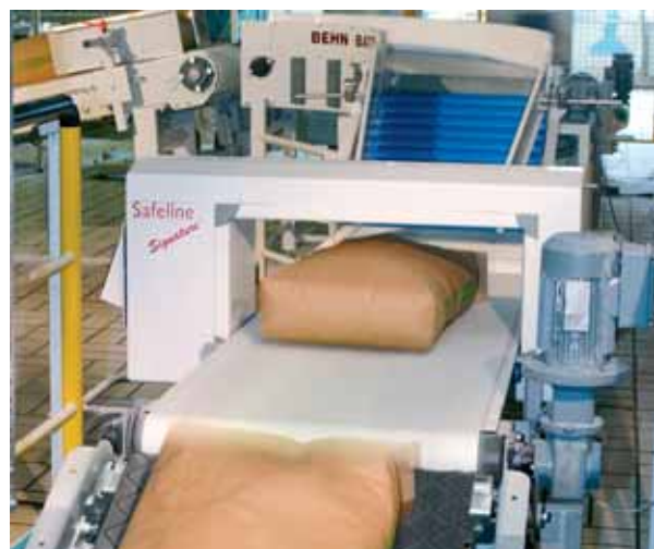
Bag transport system with metal detector
