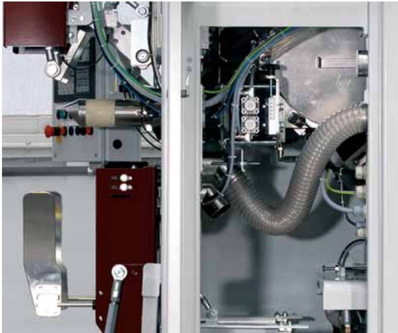
Interior view of the impeller packer with vertical filling impeller and pinch valve dosing especially for the food industry
