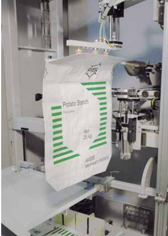
Suction bar to take the empty bag out of the bag magazine
