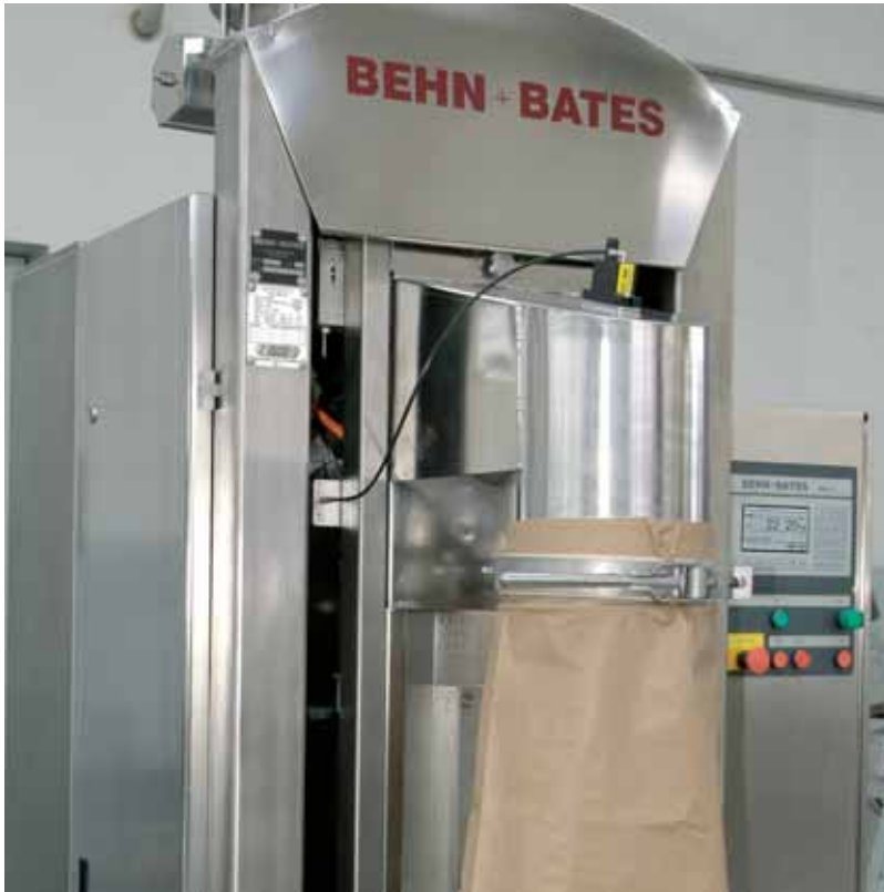
Auger packer made of stainless steel with filling spout for open mouth bags
