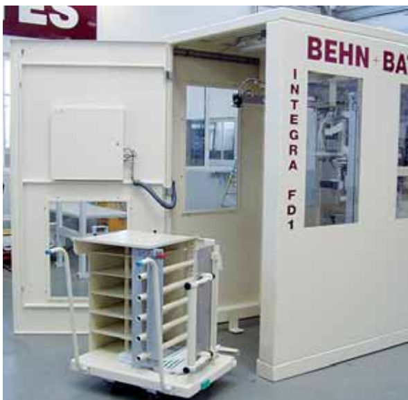
Rapid-change bundle magazine carriage for a capacity of up to 200 bags
