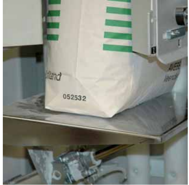
Bag chair provided as bag guiding plate for the smooth bag discharge
