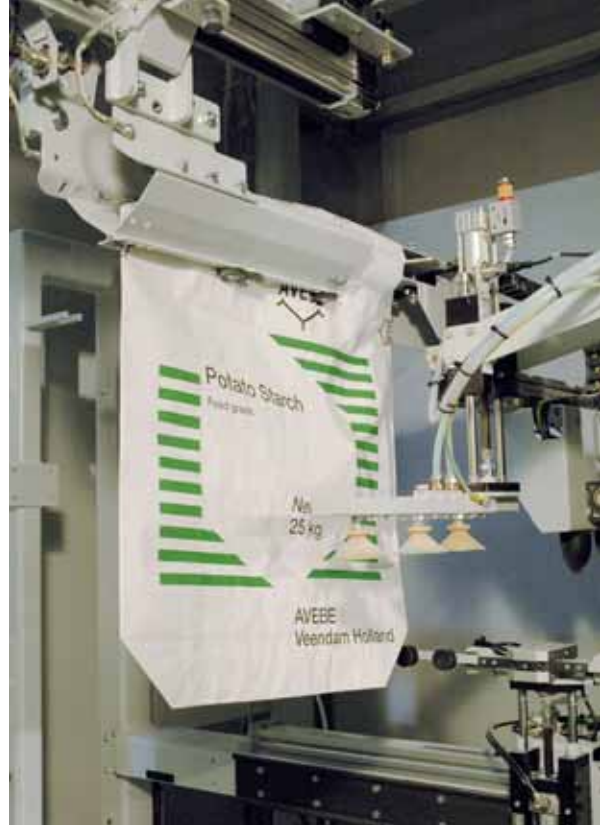
Stretching cone (within the valve) for the optimum valve opening and trouble-free empty bag application
