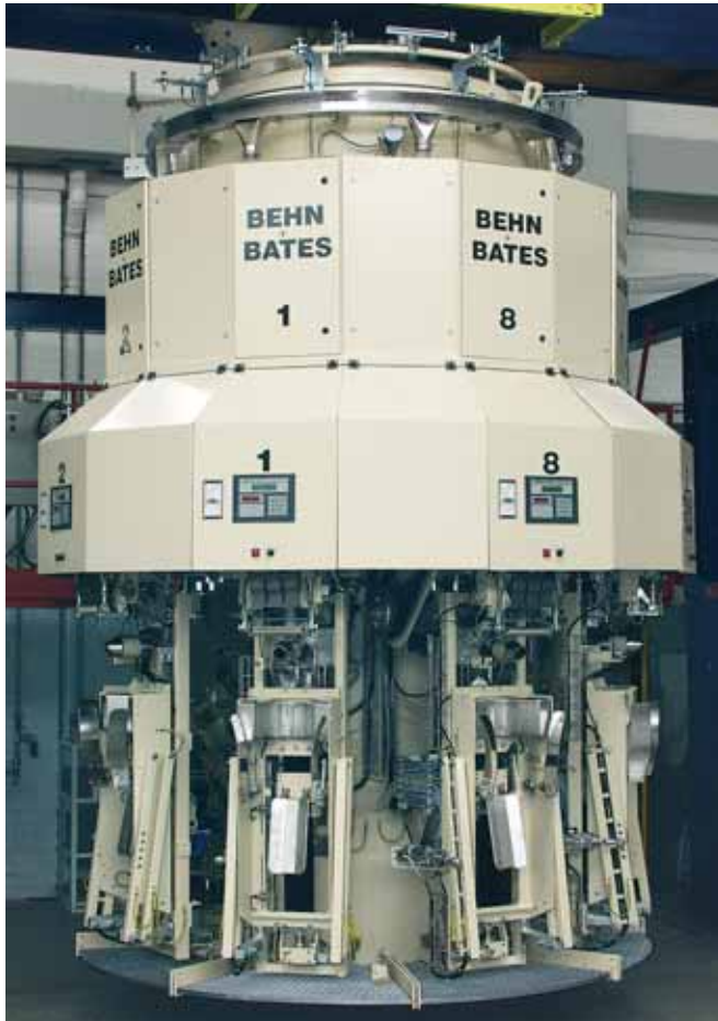
8-spout ROTOSEAL system based on the impeller filling principle for starch
