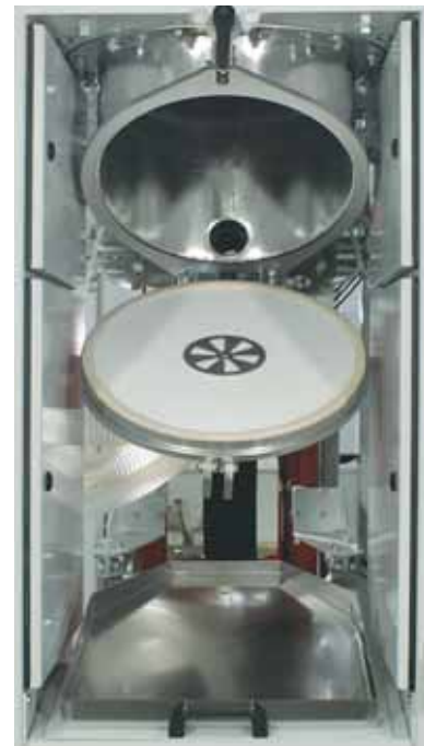
Opened filling chamber bottom for quick and easy cleaning
