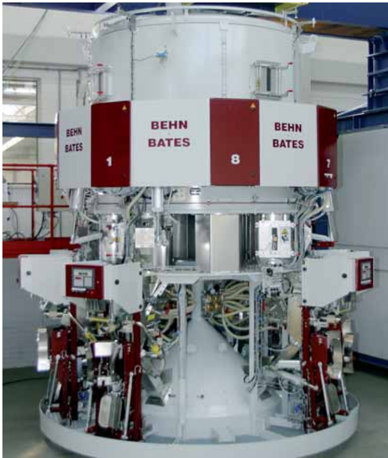
Air type ROTOSEAL system – can be extended from 6 to 8 spouts –
