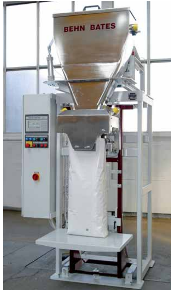
Gravity packer with filling spout for open mouth bags
