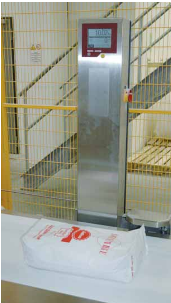
Belt control and check weigher
