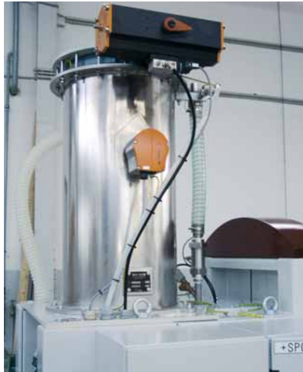
Filling chamber in electropolished stainless steel design
