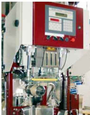
Filling spout with integrated sealing station
