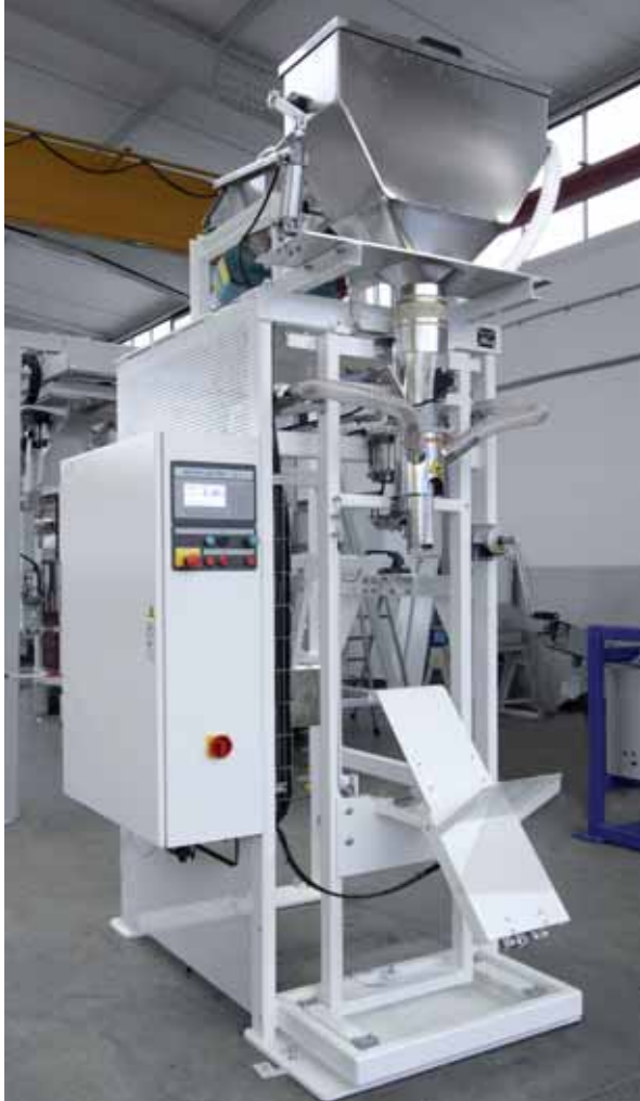
Gravity packer with vertical filling tube
