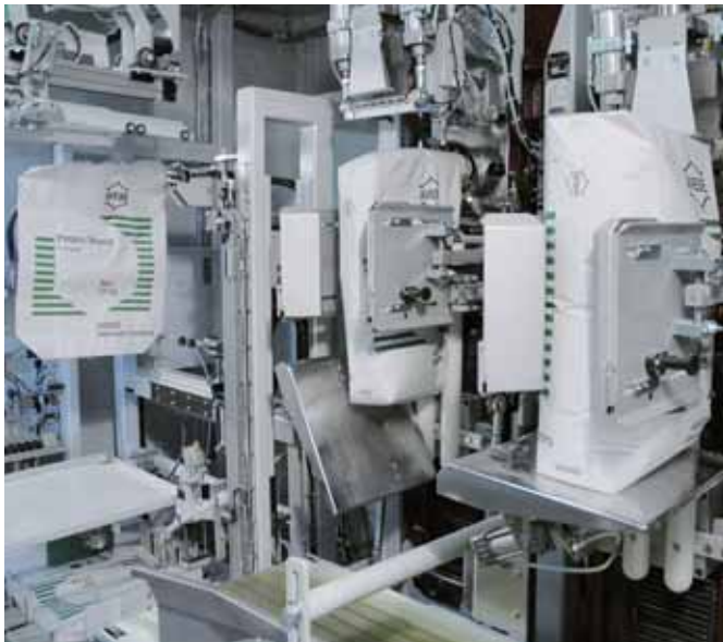
INTEGRA in operation: applying, filling and sealing
