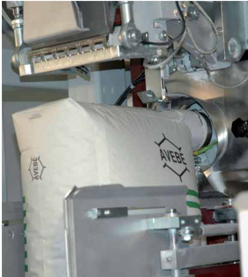
Valve bag sealing station – space- and cost-saving integration at the filling spout
