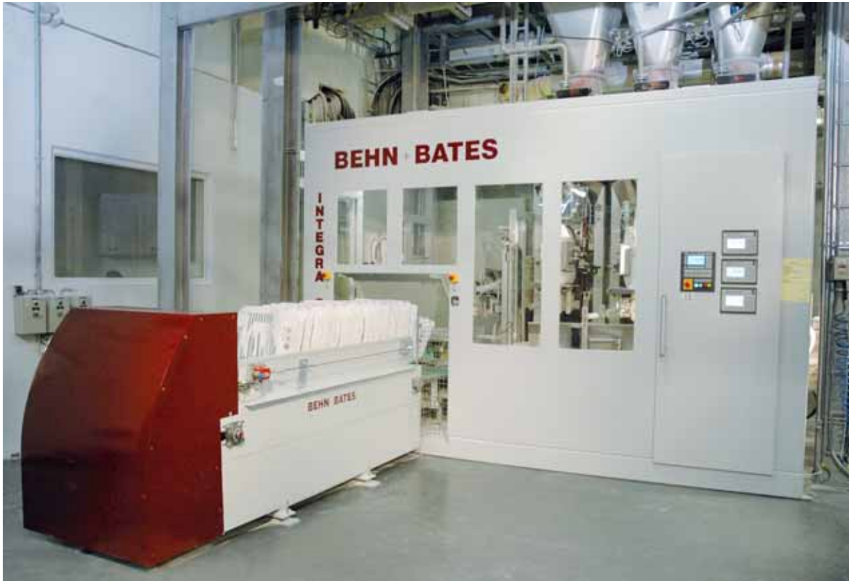
INTEGRA FD3 for the filling of starch at an output of 600 bags per hour
