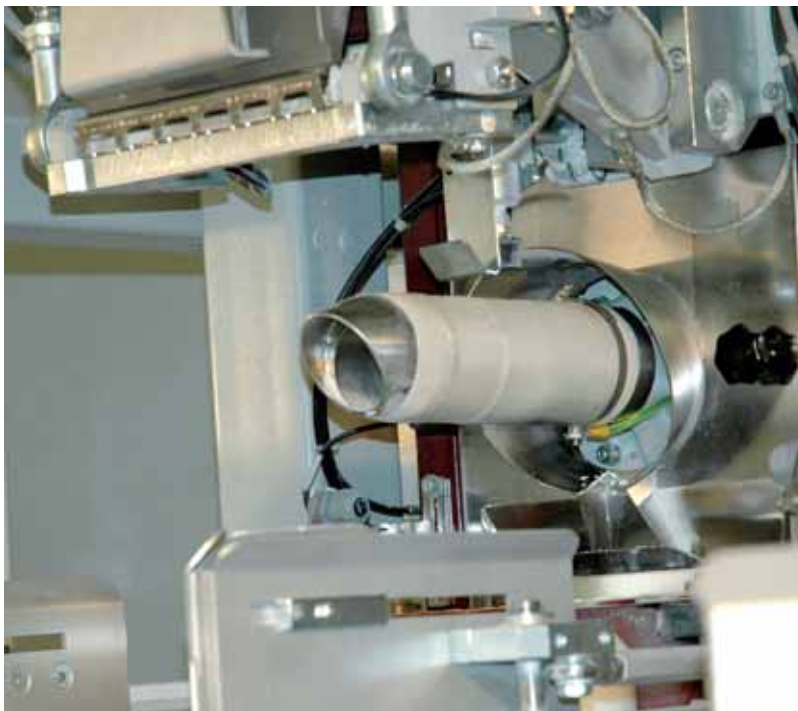
BEHN + BATES filling nozzle with inflatable sleeve for the clean product filling and above-installed ultrasound sealing station for the hermetic sealing of the filled valve bag
