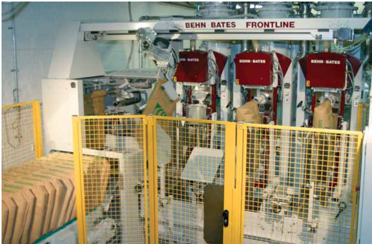
3-spout filling machine for sugar, installed in a West German sugar factory
