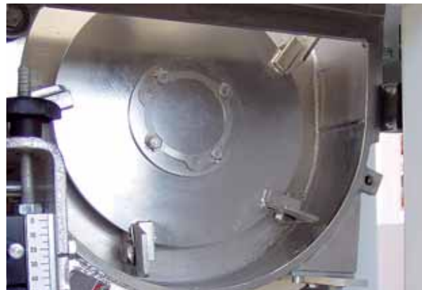
Vertical filling impeller
